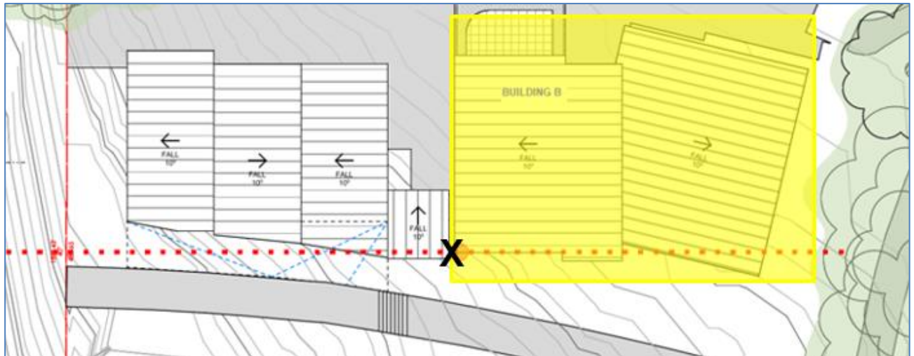
Figure 9 Height of Building B, to be measured at point “X”.
